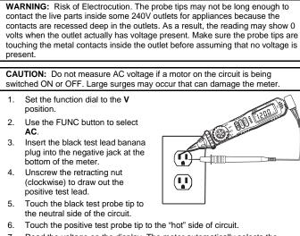
Read the voltage on the display. The meter automatically selects the optimum range or the user may manually select a range using the RANGE button.
