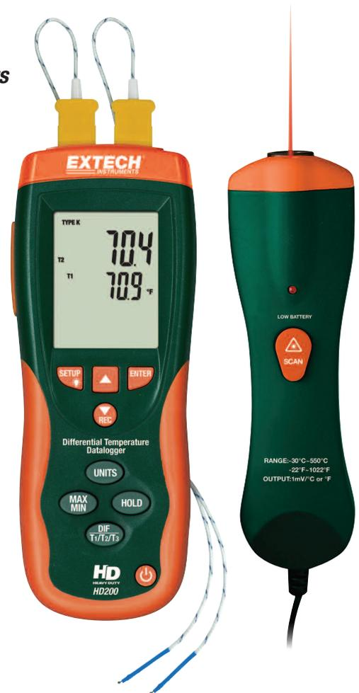
Take differential temperature readings with dual Type K thermocouple probes. Shown above with bead wire Type K thermocouple probe (included) and optional TP200 Type K Pipe Clamp Probe.
