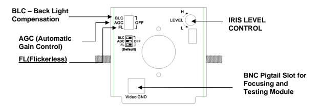
b. Front panel design (For Fixed Lens Model)
