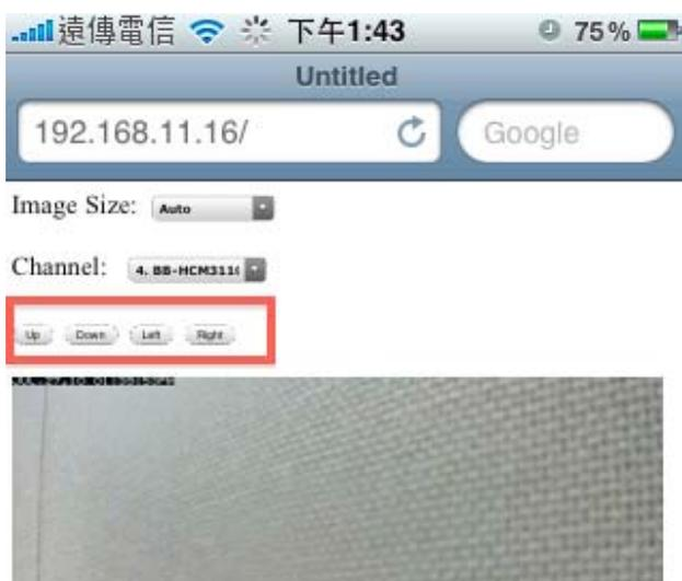
If a PTZ camera is selected, the corresponding control buttons will display (control PT only)
