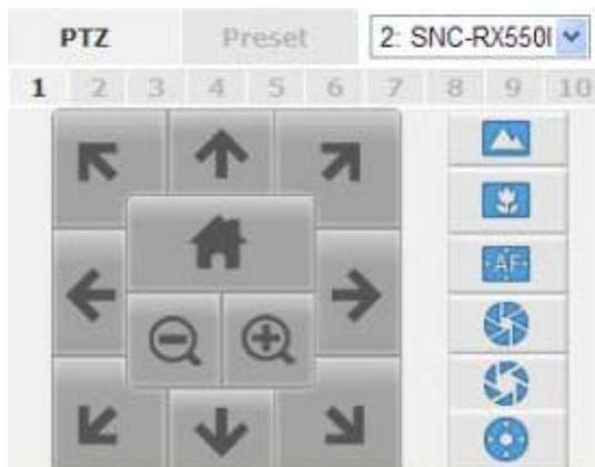
PTZ control provides functions to pan, tilt, and zoom a PTZ camera as well as the ability to adjust camera focus and iris.
