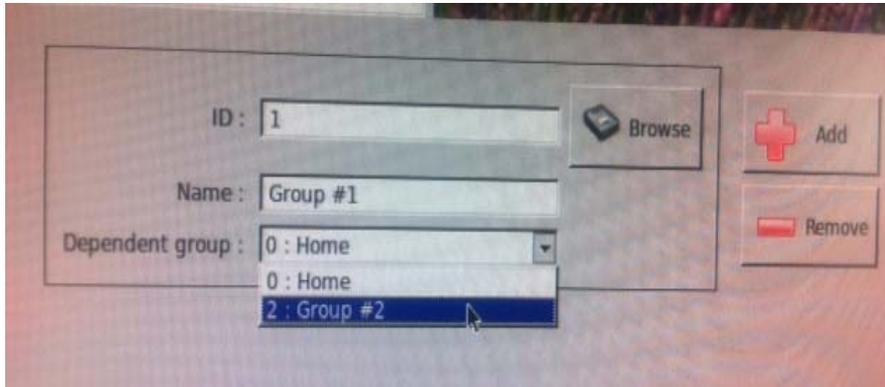
Or you can move a camera or a sub-group to a new one by using the "Dependent group" option at the bottom.
