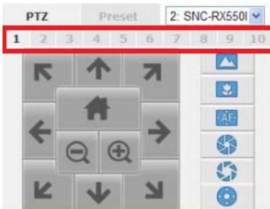
The bar highlighted above controls the moving angle. Larger number means bigger movement angle.
