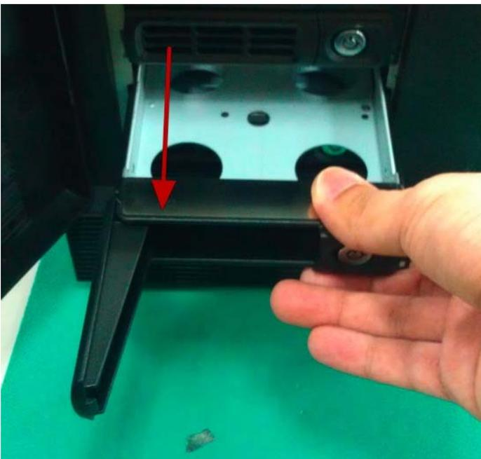
Pull the HDD tray out of the case.
