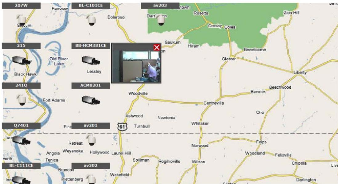
When the NVR receives an event triggered from any of the cameras, their videos will be displayed on the Local-Map and you can double-click on the video to enlarge it.
