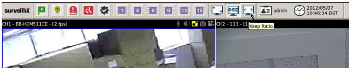
You can change this and display the video in its original aspect ratio by using the "Keep ratio" function from the right-click menu, or the top of the video if OSD is enabled. This will make the video of that particular channel to be displayed in its original aspect ratio.
