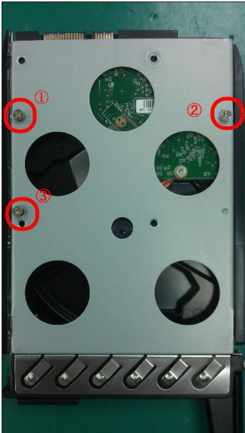
Place the HDD in the tray and secure it with three flat head screws at the bottom of the tray.
