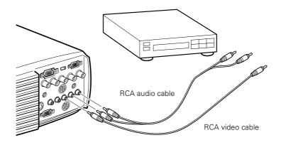
If you'll be using audio, connect the RCA audio cable to the left and right Audio ports of the projector (insert the white plug into the L port and the red plug into the R port). Connect the plugs at the other end of the cable to the audio output ports of the video source.
