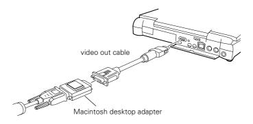
4. Tighten the screws on the connectors.
