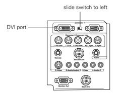
2. Using the tip of a pen or a small screwdriver, slide the DVI/VGA interface switch to the left. (If you need to use the projector's VGA port again, be sure to slide the switch back to the right.)
