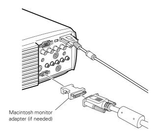
6. Tighten the screws on the connectors.
