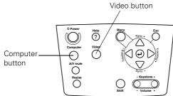
These buttons switch the display between the video source(s) and the computer source(s).
