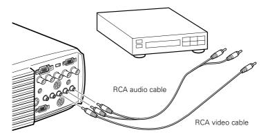
2. If you'll be using audio, connect the RCA audio cable to the left and right Audio ports of the projector (insert the white plug into the L port and the red plug into the R port). Connect the plugs at the other end of the cable to the audio output ports of the video source.
