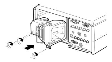
Tighten the screws on the new lamp.
