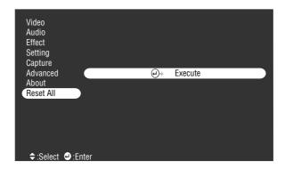
Select Reset All and press the Enter button on the control panel or remote control to display the confirmation screen. Select Yes to reset all the default settings or No to cancel.
