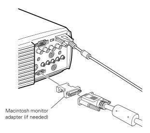
6. Tighten the screws on the connectors.
