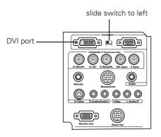
Using the tip of a pen or a small screwdriver, slide the DVI/VGA interface switch to the left. (If you need to use the projector's VGA port again, be sure to slide the switch back to the right.)
