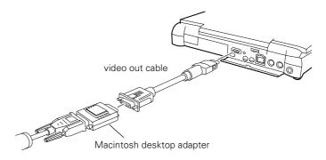
4. Tighten the screws on the connectors.
