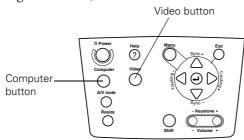
These buttons switch the display between the video source(s) and the computer source(s).
