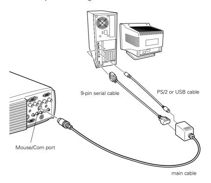
1. Connect the round end of the main cable to the projector's Mouse/Com port, as shown.
