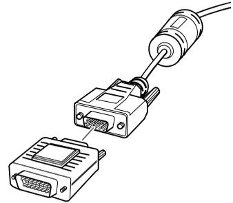
4. Tighten the screws on all the connectors.
