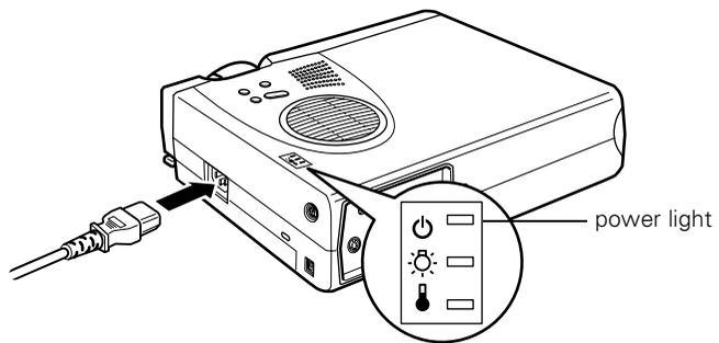
2. Plug the other end of the cable into a grounded electrical outlet.
