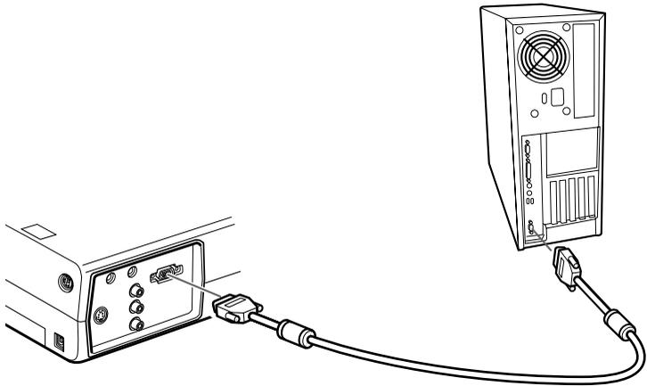
4. Tighten the screws on all connectors.
