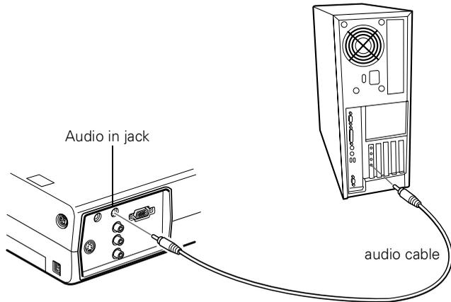
2. Connect the other end of the audio cable to the speaker or audio out port on your computer's sound card.
