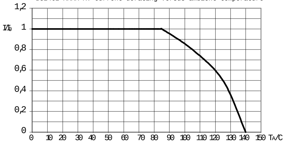
B82462-XXXX-X: current derating versus ambient temperature
