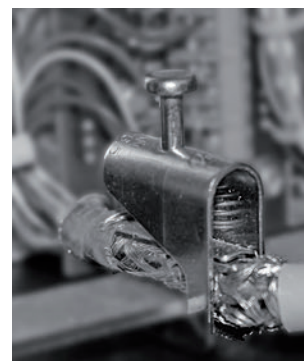
Fig. 2-17: Shield connector terminal with cable
