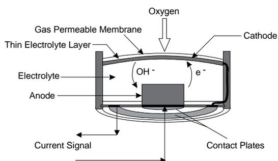
Fig. 3.9 Trace Oxygen sensor design principle
