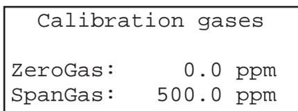
In the CALIBRATION GASES menu, the values for zero and span gas should be entered: these values should be taken from the gas supplier's certification. Values must be correctly set for results to be accurate. In multi-channel units, the values for each channel must be entered separately.
