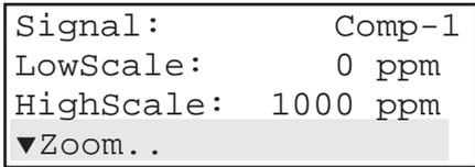
The “Signal” parameter defines the value to be sent to the selected output. The following options (partly dependent on the number of measuring channels and sensors installed) are available:
