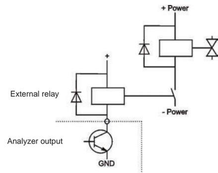
Fig. 4-31: Driving high-current loads
