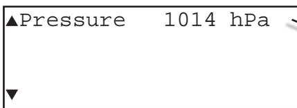
Displays the current pressure, either from an internal or external sensor or manually entered.
