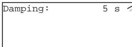
The time for the electronic signal damping is entered here.
