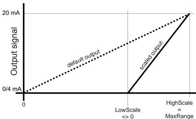
The “LowScale” and “HighScale” parameters allow a concentration value to be set to correspond to the lower (0 or 4 mA) or upper signal value (20 mA). The limits for these parameters are given by the "MinRange" and "MaxRange" parameters, specifying the physical measuring ranges of each instrument (👉 5.7.4.1, page 5-27).
