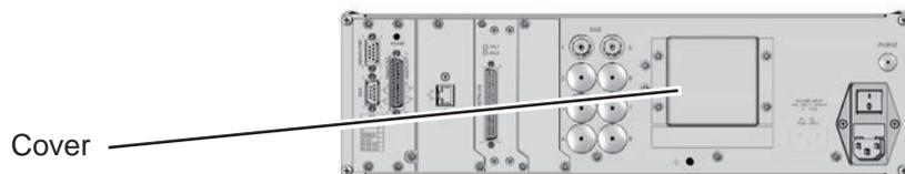
*Fig. 3.10 Cover for tO<sub>2</sub> sensor block at rear panel*
