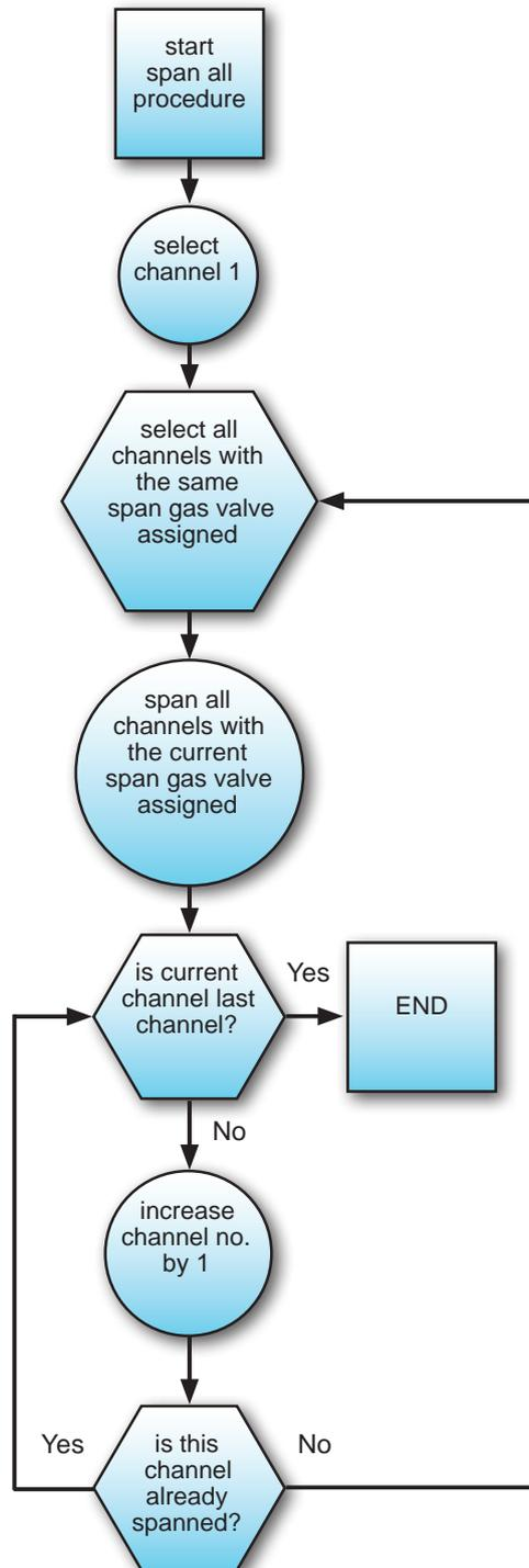
Fig. 7-5: Span All Calibration Procedure Flow Diagram
