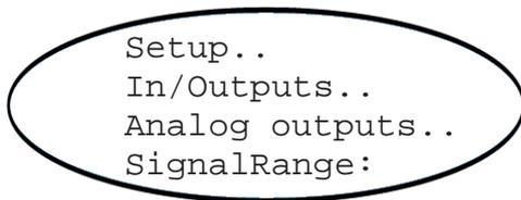
The signal range for the analog outputs is set via the signal "Range" parameter.
