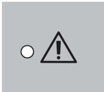
“Failure” is indicated when this red LED is lit.
