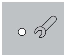
A flashing red LED in the middle indicates “Maintenance request”, “Function check” or “Off-spec operation”.
