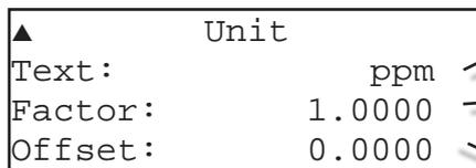
If necessary, an offset to be added to the measured value can be set here.
