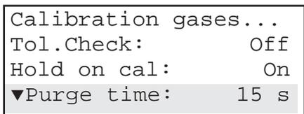
Last but not least valve supported calibration procedures require a purge time to be specified:
