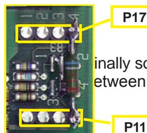
Initially solder in the resistor between P11/ P17.
