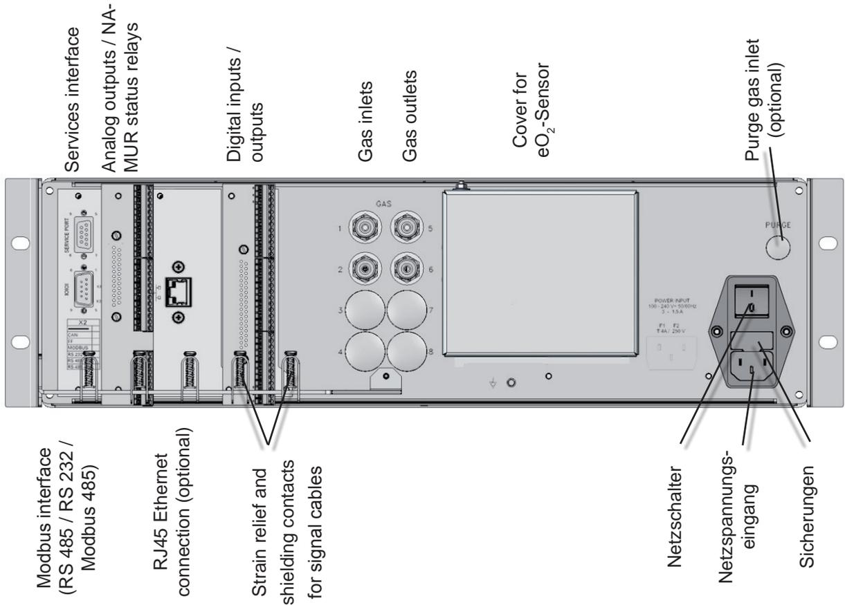
Fig. 4-12: X-STREAM X2GP - Rear panel, with terminal adapters and brackets for rack mounting
