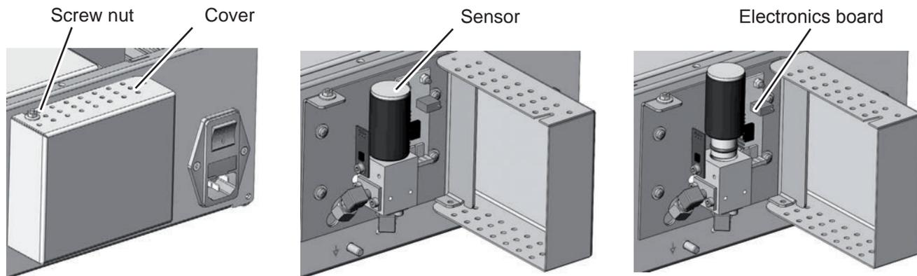
1. Loosen the screw nut at the cover's upper side.
