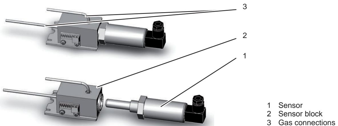
Fig. 3-14: Trace Moisture Sensor Assembly
