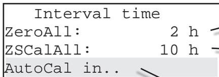
Sets the time between two zero calibrations in autocal mode.
