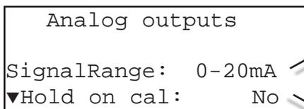
This line sets the output signal range for all outputs.
