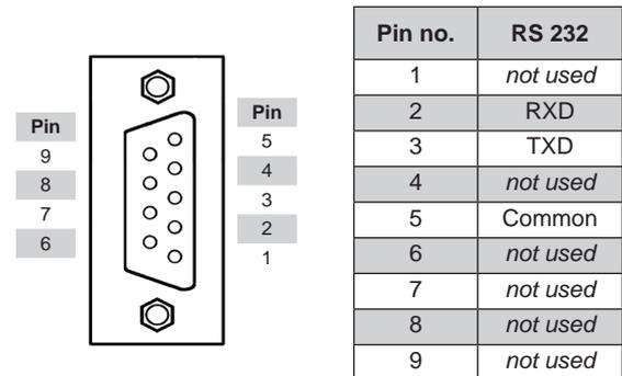
Fig. 7-18: Service Port Connector - Serial RS 232 Interface
