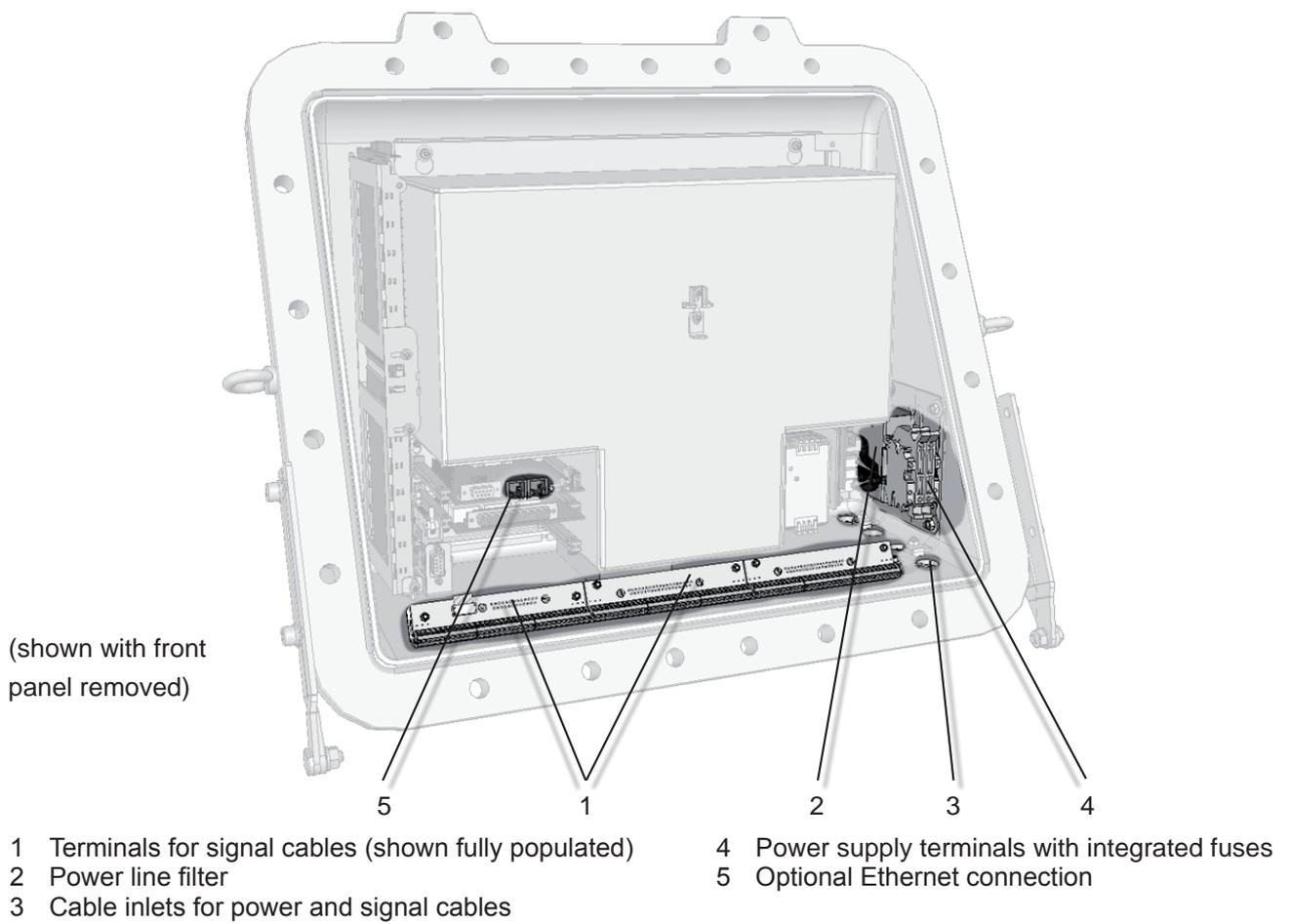
*Fig. 1-14: X-STREAM X2FD - Terminals*
