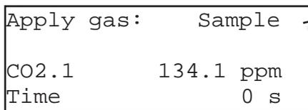
Use the **↑** and **↓** keys to switch between **Sample, Zero, Span** and **None**.
