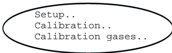
Starting from the measurement screen press the DOWN key to open the MAIN MENU, enter the SETUP-CALIBRATION.. menu and directly enter the CALIBRATION GASES.. menu.
