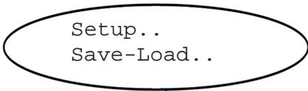
Starting at the measurement screen press the DOWN key to open the MAIN MENU, enter the SETUP and next the SAVE-LOAD.. menu.
