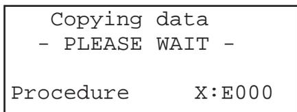
The instrument now stores the currently used (and changed by operator) analyzer setup into a special memory area. This data is then called **UserData** and used for backup only, while the data used for operation still is **CfgData**.
