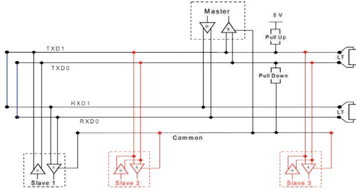
Figure 22 : Changing a 4-Wire cabling system into a 2-Wire cabling system
