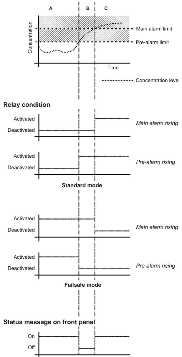
Fig. 5-3: High Pre-Alarm and Main Alarm
