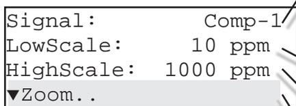
This line determines which concentration value corresponds to the lower signal limit (0 or 4 mA).
