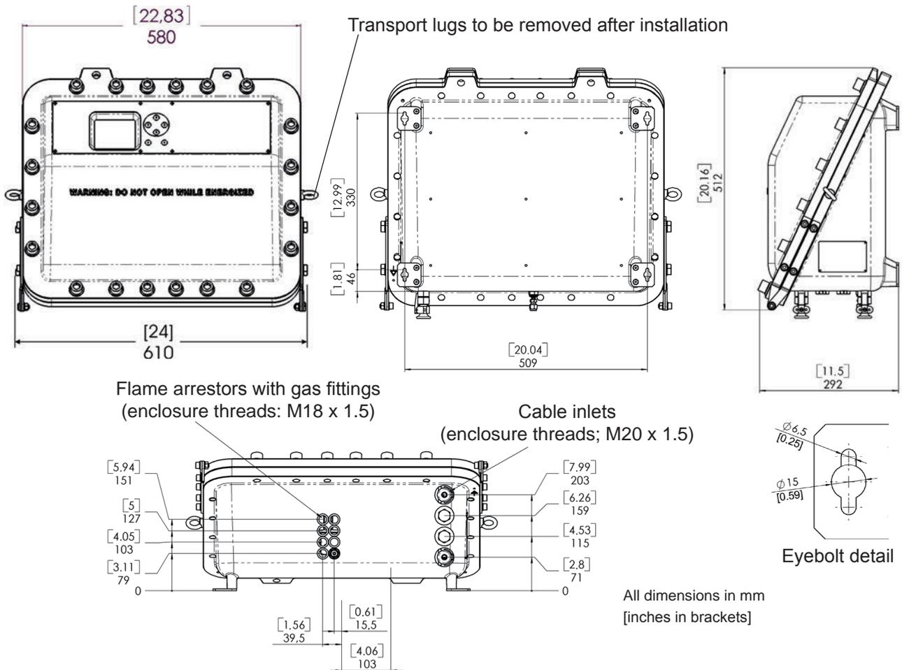
Fig. 2-12: X-STREAM X2FD - Dimensions
