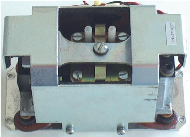
This instruction explains the procedure to replace the diaphragms of sample gas pumps (PN 42716569) used in the X-STREAM series gas analyzers.
