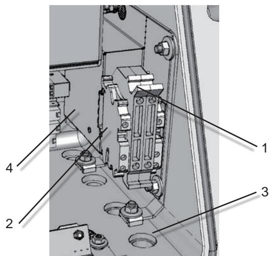
Fig. 2-13: X-STREAM X2FD - Power Supply Terminals / Fuse Holders
