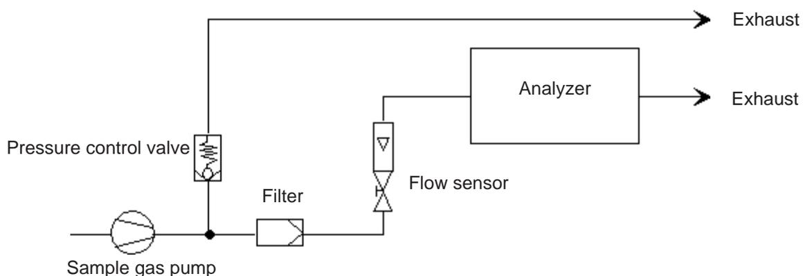
Fig. 4-3: Installation in bypass mode
