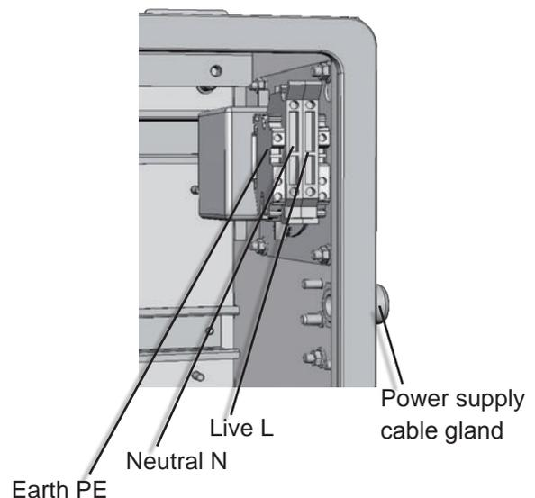
Fig. 4-25: Power supply connections
