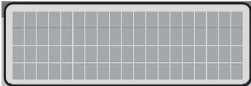
The display has 4x20 characters, either liquid crystal or vacuum fluorescent (LCD or VFD).
