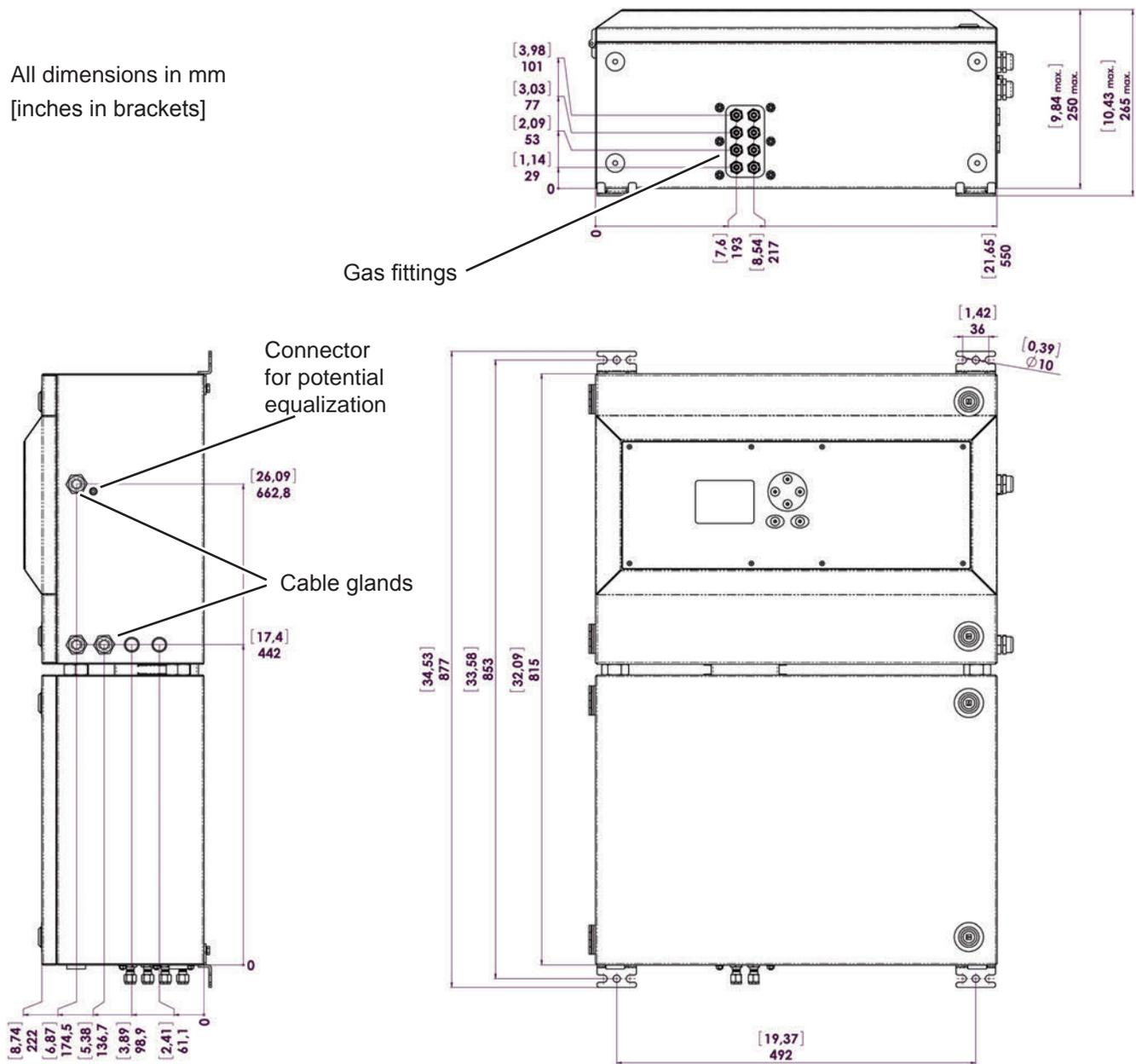
Fig. 2-9: X-STREAM XXF - Dimensions
