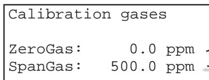
Enter the concentration value for the zero gas to be used during zero calibration.
