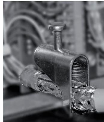
Fig. 4-29: Shield connector terminal with cable
