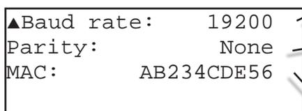
MAC ID of the Ethernet port (visible only if "Interface" is set to **Ether**)
