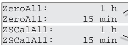
The first two lines allow to enter a time to elapse from the current moment, before the next zero calibration for all channels is started. Preset is the remaining time until the next zero calibration starts.
