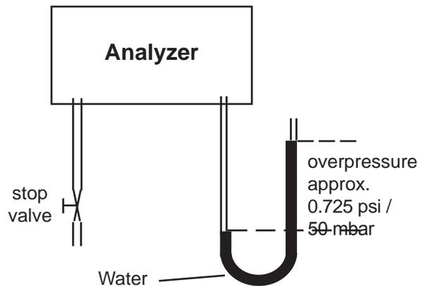
Fig. 7-1: Leak Testing With U-Turn Manometer
