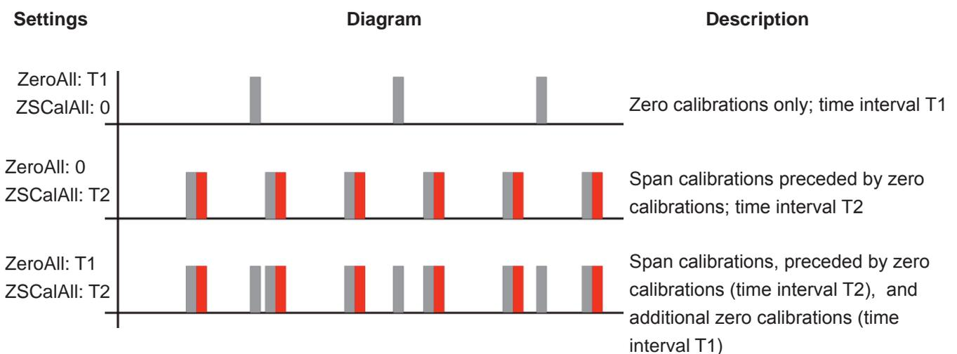
Fig. 7-8: Graphical Explanation of Interval Time Settings
