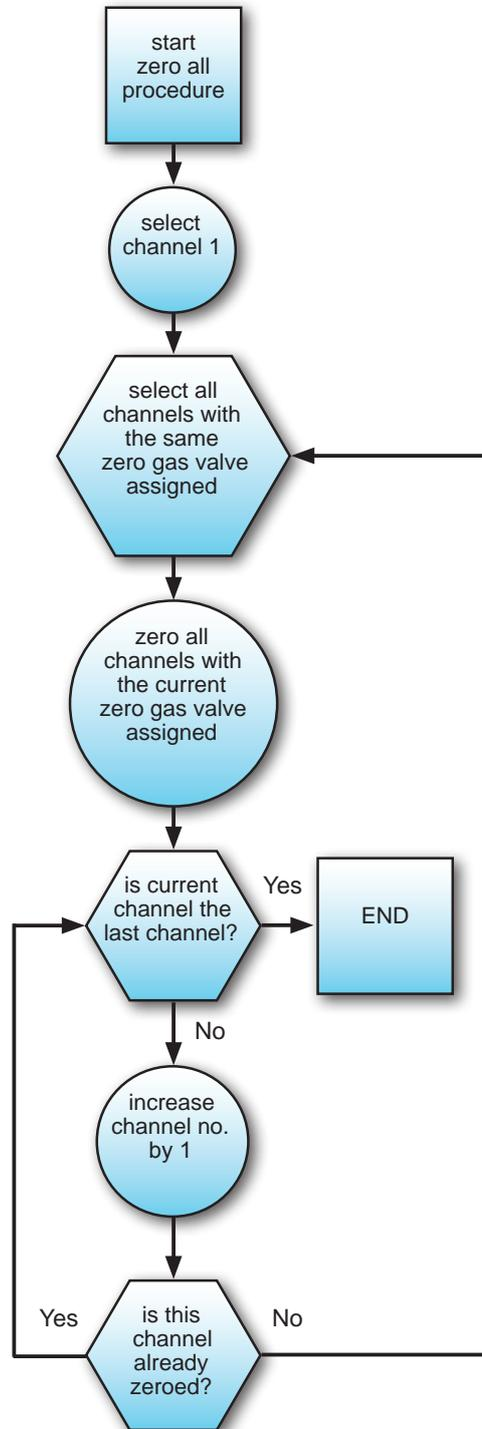
Fig. 7-4: Zero All Calibration Procedure Flow Chart
