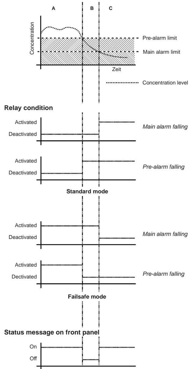
Fig. 5-4: Low Pre-Alarm and Main Alarm
