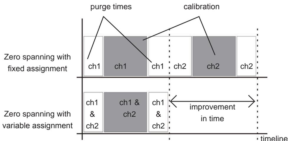
Fig. 7-2: Calibration Improvement by Variable Valve Assignments
