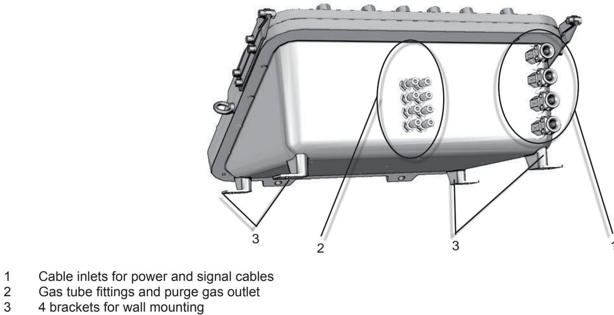
Fig. 1-13: X-STREAM X2FD - Bottom View
