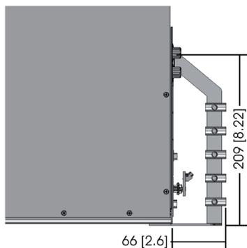
Strain relief bracket, detail (model with clamping adapters)
