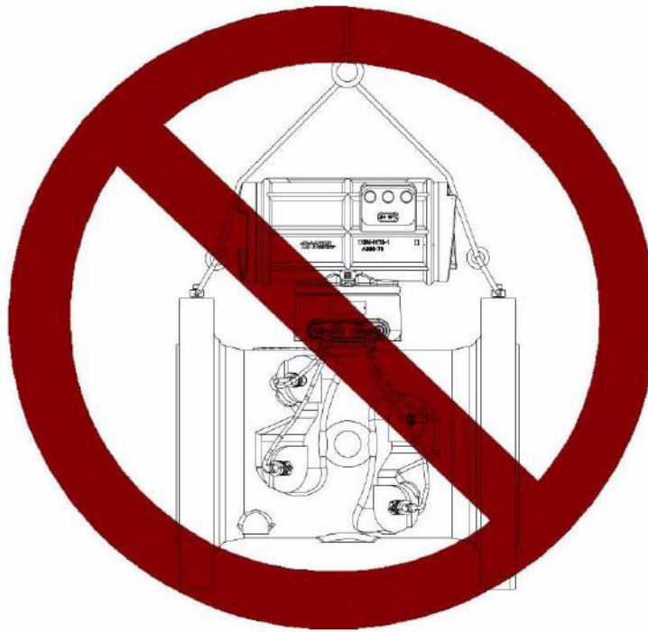
Figure 3-4 Incorrect Sling Attachment
