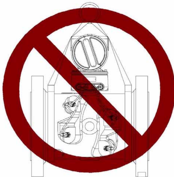
Figure 3-6 Incorrect Sling Attachment
