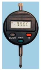
This electronic indicator combines the ease of digital reading with the applications of standard plunger dial indicators. Dial diameter 60mm, with 8mm stem and lug back mounting. 3 button operation: on/off switch, imperial/metric conversion.
