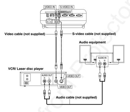
Use common RCA cables (not provided) to connect your VCR, laser disc player or document camera to your projector. To make these connections, simply:
