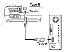
NOTE: Wait at least 5 seconds after disconnecting the USB cable before reconnecting it and vice versa. The computer may not identify the built-in mouse receiver if it is repeatedly connected and disconnected in rapid intervals.
