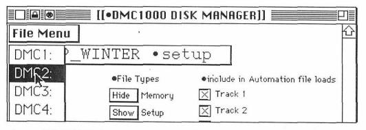
Selecting a DMC1000 from this menu will cause the contents of the disk's file directory to be sent to Project Manager. If a different disk is inserted in the DMC1000's floppy disk-drive, use this menu again to access the contents of the new disk's file directory.
