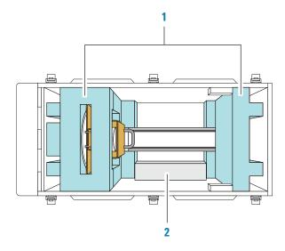
**3** While holding the handle on the shipping brace and supporting the robot under the mast, carefully lift the robot out of the crate.
