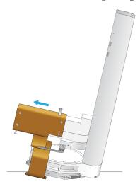
**6** While holding the brace by the handle, carefully slide the brace away from the robot.
