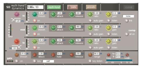
All hannels can have their Dynamics (Compressor) modules switched into Multi-band mode
