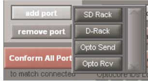
The simplest way to set up a system is to automatically Conform All Ports and all relevant Ports will be created. However, Ports can be manually added and removed using the Add Port and Remove Port buttons. Pressing the Add Port button provides a list of Port types to choose from. There are different rack types and also Opto Send and Receive Ports.
