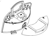
to attach the antenna to the four tabs on the back of the Delphi Premium Sound System. Or you can extend the entire 20' cable away from the system to improve reception. To reattach the top cover, line up all tabs and then slide the cover toward the front of the unit until a click is heard. Make certain that all tabs are engaged and the rear of the panel is aligned with the rear cover.
