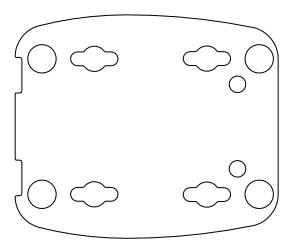
Photocopy this diagram of the screw-locator pattern on the bottom of your XM Antenna to use as a template for wall attachment.
