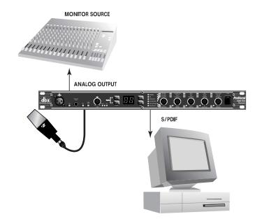
This application allows you to send a digital signal to a receiving device (such as a DAW or digital recorder) and route the analog signal to a monitoring device (such as a mixer or headphone amplifier) simultaneously.
