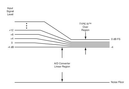
Figure 2 - Input Signal Levels Mapped to Type IV Over Region
