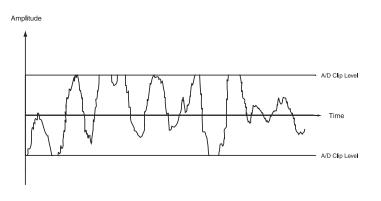
Figure 3b - Signal of Fig. 3a Going Beyond the A/D Clip Level
