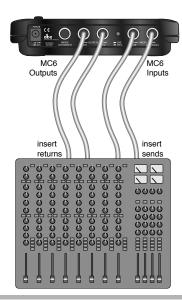
Use the MC6 to compress those pesky individual tracks by inserting it in the insert path of your mixer for a single channel or for a (stereo) linked pair of signals.
