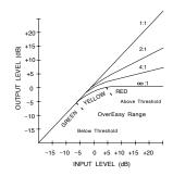
Figure 1: Hard Knee Compression Curve, and Threshold LEDs.
