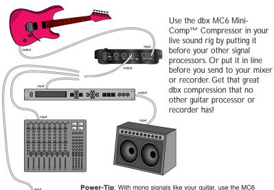
**Power-Tip:** With mono signals like your guitar, use the MC6 as a Y-cable. Both outputs send the same signal when the mono input is used as the only input. This means you can send signal to a recorder AND to an amp/speaker system independent of each other.
