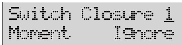
• Note that the underscore indicates the currently selected parameter for editing. To select parameters to edit from the current page, simply press the **DATA** wheel until the underscore is under the parameter that you wish to edit.
