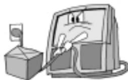
Do not cover the top of the television set. Ventilation will be prevented, and it may be a cause of fire if the product is internally overheated.
