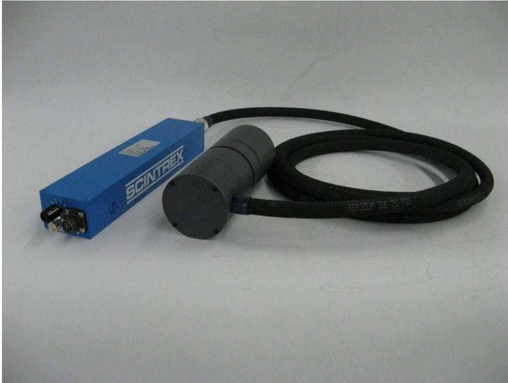
Figure 17 – the CS-L Sensor Head and Electronics
