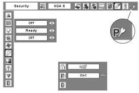
When the projector is locked with a PIN code, the PIN code lock symbol appears on the menu bar.
