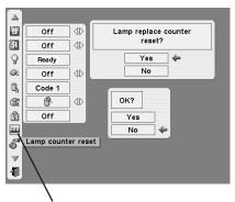
Move the pointer to Lamp counter reset and then press SELECT button. The message "Lamp replace counter reset?" is displayed.
