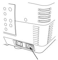
Connect AC Power Cord (supplied) to a projector. AC outlet must be near this equipment and must be easily accessible.
