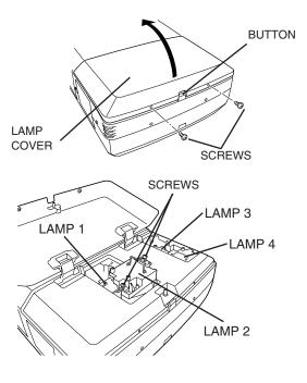
Make sure which number of lamp needs to be replaced on Lamp Status Display. Figure shows case of replacing LAMP 2.
