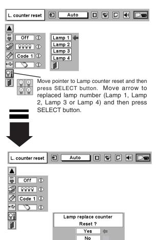
Message "Lamp replace counter Reset?" is displayed. Move pointer to [Yes] and then press SELECT button.
