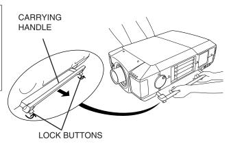
Pull up lock buttons to release lock.
