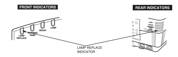
Allow a projector to cool, for at least 45 minutes before you open Lamp Cover. The inside of a projector can become very hot. For continued safety, replace with a lamp assembly of the same type.
