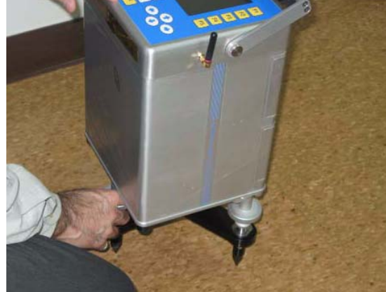
Figure 3-7 - Leveling the Tripod using the Front Footscrew
