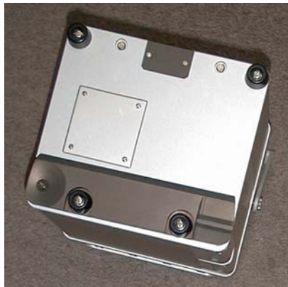
Figure 5-6 - Bottom of Autograv Slider Plate. The slider plate is the horizontal grey plate with a cone and vee-groove and two screws shown above.
