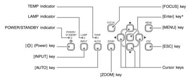
\* The projector's enter key does not have anything printed on it. When you see [ENTER] in this manual, it means you should press the projector's enter key or the [ENTER] key of the remote controller.
