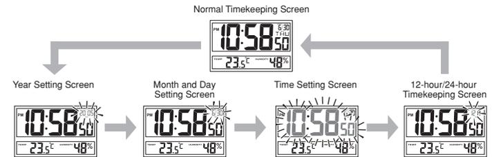
2. While the screen you want is displayed, use the **+** and **-** buttons (①) to change the flashing digits.
