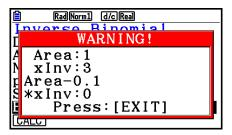
The calculation results of Inverse Binomial Cumulative Distribution are integers. Accuracy may be reduced when the Area value has 10 or more digits. Note that even a slight difference in calculation accuracy affects calculation results. If a warning message appears, check the displayed values.
