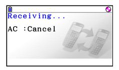
The calculator enters a data receive standby mode and waits for data to arrive. Actual data receive starts as soon as data is sent from the sending calculator.
