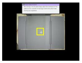
When the document camera is positioned correctly, position adjustment will end and the dialog box will close. At this time the monitor screen (the image being picked up by the document camera) will be projected.
