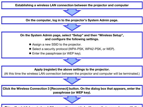
This will establish a wireless LAN connection provided with security in accordance with the selected protocol.
