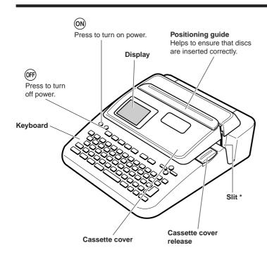
\* The right end of the slit becomes a "tape outlet" when a tape cartridge is loaded in the printer.
