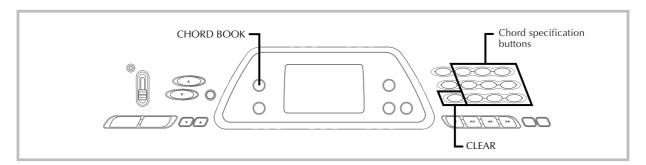
The Chord Book feature of this keyboard makes it possible for you to look up information about chords quickly and easily. Simply input the name of the chord and the keyboard keys you should press, the fingers you should use, and the notes that make up the chord appear on the display along with the chord name.
