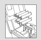
When using the P-touch labeler with batteries, insert six new AA alkaline batteries (LR6), making sure that their poles point in the correct directions. Always replace all six batteries at the same time using brand new ones.
