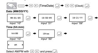
You can also confirm the figure and move to the next setting by using the right cursor key
