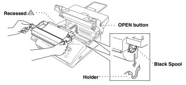
**6** Press down on both sides of the cover to close it securely.
