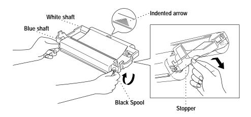
**3** Turn the black spool on the right clockwise to tighten the ribbon, as shown.
