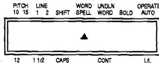
**When you switch the machine on, the Word Spell is automatically switched on.**
