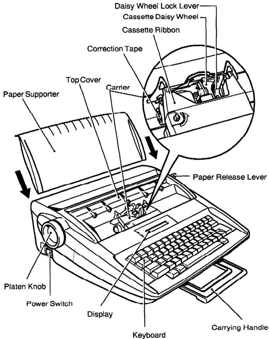
**Paper release lever:** Pushing this lever loosens tension on the paper so that it can be adjusted as necessary.
