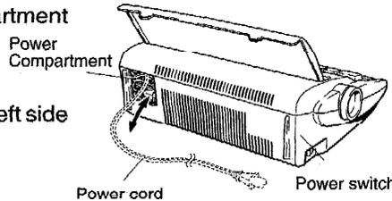
The power switch is located on the left side of the typewriter near the rear.
