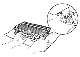
4 Put the toner cartridge back into the drum unit until you hear it lock into place. If you put it in properly, the lock lever will lift automatically.
