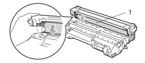
4) When you find the substance on the drum surface that matches the print sample, gently dab the surface of the OPC drum with a cotton swab that is lightly dampened with isopropyl alcohol.
