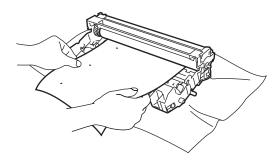
3 Turn the white gear on the drum as you check the surface of the OPC drum (1).
