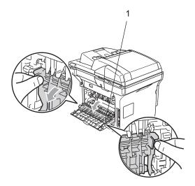
5 Using both hands, gently pull the jammed paper out of the fuser unit.
