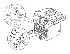
2 Hold down the lock lever on the right and take the toner cartridge out of the drum unit.
