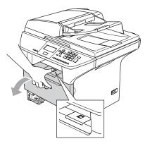
4 Slowly take out the drum unit and toner cartridge assembly. The jammed paper may be pulled out with the toner cartridge and drum unit assembly, or this may release the paper so you can pull it out of the paper tray opening.
