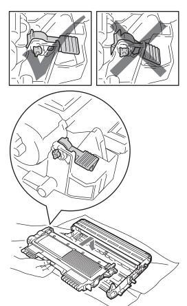
8 Clean the primary corona wire inside the drum unit by gently sliding the green tab from left to right and right to left several times.
