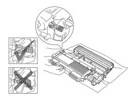
6 If you were able to remove the drum unit and toner cartridge assembly and the jammed paper, you have cleared the paper jam. Put the drum unit and toner cartridge assembly back into the machine and close the front cover. If the machine does not start printing automatically, press **Start**.
