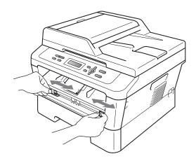
5 Using both hands, put one sheet of paper or one envelope in the manual feed slot until the front edge of the paper or envelope touches the paper feed roller. When you feel the machine pull in the paper, let go.
