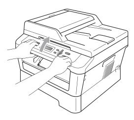
You can still use the machine while the scanner cover is up. To close the scanner cover, push it down with both hands.
