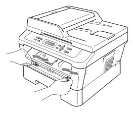
4 Using both hands, put one sheet of paper in the manual feed slot until the front edge of the paper or transparency touches the paper feed roller. When you feel the machine pull in the paper, let go.
