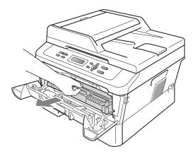
4 Push down the green lock lever and take the toner cartridge out of the drum unit.
