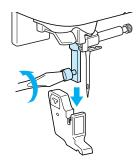
Position the free-motion echo quilting foot "E" on the left side of the presser bar with the holes in the quilting foot and presser bar aligned.
