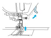
Press the black button on the presser foot holder to remove the presser foot.
