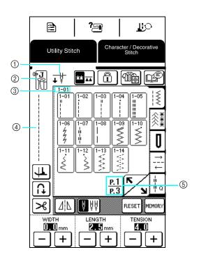
① Shows whether the machine is set for a single needle or twin needle, and the needle position when the machine is stopped. The desired needle position can be set (see page 20).
