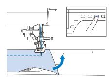
The pivot setting is useful when changing the sewing direction. When the machine is stopped at the corner of the fabric, the machine stops with the needle in the fabric and the presser foot is automatically raised so the fabric can easily be rotated ("Pivoting" on page 84).
