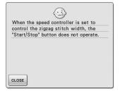
This message is displayed when the speed control lever is set to control the zigzag stitch width, and the "Start/ Stop" button is pushed. Use the foot controller to operate the machine.
