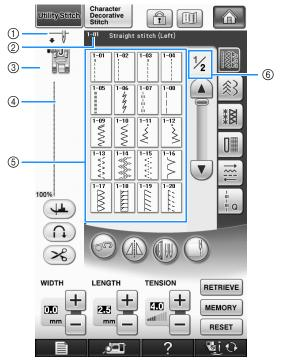
① Shows single or twin needle mode setting, and the needle stop position.
