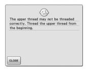
This message is displayed when it seems that the upper thread has not been threaded correctly.
