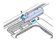
Insert a wound bobbin into the machine. (see page 54 for Setting the bobbin.)
