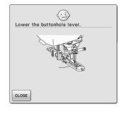
This message is displayed when the buttonhole lever is up, a buttonhole stitch is selected, and the "Start/ Stop" button or "Reverse/ Reinforcement Stitch" button is pushed.
