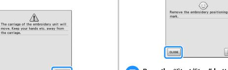
→ The built-in camera automatically searches for the embroidery positioning sticker, and then the carriage is moved so that the center of the embroidery pattern is aligned with the center of the embroidery positioning sticker. Regardless of the setting selected in the machine settings screen, the brightness of the light changes to "5" while the builtin camera searches for the embroidery positioning sticker.
