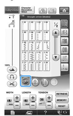
→ The key appears as , the quilting foot is raised to the necessary height, then the feed dogs are lowered for free motion sewing.
