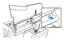
Insert the spool stand onto the notches of the machine.
