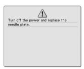
This message is displayed when you try to sew with a stitch other than a middle needle position stitch while the single-hole needle plate is installed.
