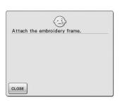
This message is displayed when the machine is ready to sew an embroidery pattern, and the "Start/Stop" button is pushed while the embroidery frame is not attached.
