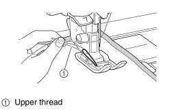
Raise the presser foot lever, and then use tweezers to pull up the bobbin thread and bring the end of the thread to the top of the fabric.
