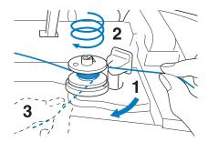
Pass the end of the thread through the guide slit in the bobbin winder seat, and pull the thread to the right to cut the thread with the cutter.
