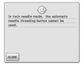
This message is displayed when the automatic needle threading button is pushed while twin needle sewing is set.
