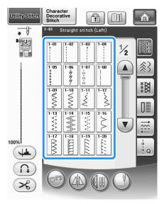
→ The symbol of the correct presser foot will be displayed in the upper left corner of the LCD screen.
