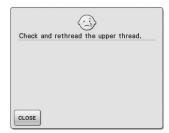
This message is displayed when the upper thread is broken or not threaded correctly, and the "Start/Stop" button or the "Reverse/ Reinforcement Stitch" button is pressed.
