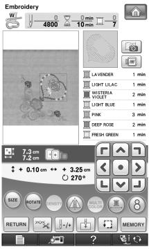
The fabric hooped in the embroidery frame can be displayed on the LCD so that the embroidery position can be easily aligned.
