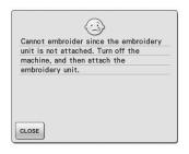
This message is displayed when the "Start/Stop" button is pushed and the machine is in embroidery mode, but the embroidery unit is not attached.
