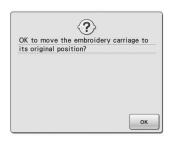
This message is displayed when replacing the embroidering bobbin thread.
