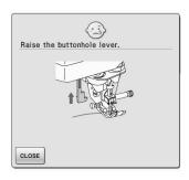
This message is displayed when the buttonhole lever is down, a stitch other than a buttonhole is selected, and the "Start/ Stop" button or the "Reverse/Reinforcement Stitch" button is pushed.
