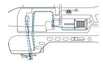
Pass the thread through the needle bar thread guides on the needle bar, then thread the needle on the left side manually.
