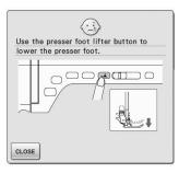
This message is displayed when a button, such as the "Start/Stop" button, is pushed while the presser foot is raised.
