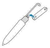
Screw the upper barrel to the tablet pen.
