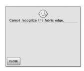
This message is displayed when the "Start/Stop" button is pressed before the edge of the fabric is detected. To detect the edge of the fabric using the built-in camera,
