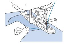
→ When sewing is completed, the machine will sew reinforcement stitches and stop automatically.
