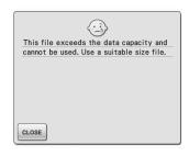
This message is displayed when the file size exceeds the data capacity of the machine.
