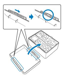
Place the lid on top of the case so that the notches in the lid align with the tabs on the case, and then slide the bar on each side back to the center of the accessory case.
