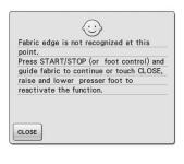
This message is displayed when the built-in camera cannot detect the edge of the fabric.
