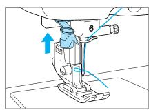
④ Simultaneously release both thread and automatic needle threader lever. The threading hook will pass the thread through the eye of the needle.
