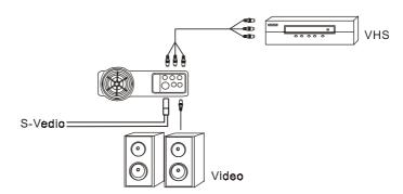
Figure 28 Connection of AV box
