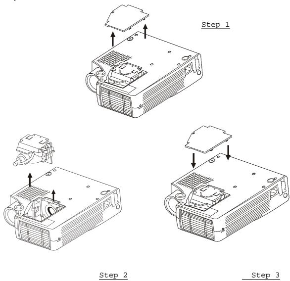
Figure 20 Lamp replacement: Step 1, Step 2, Step 3
