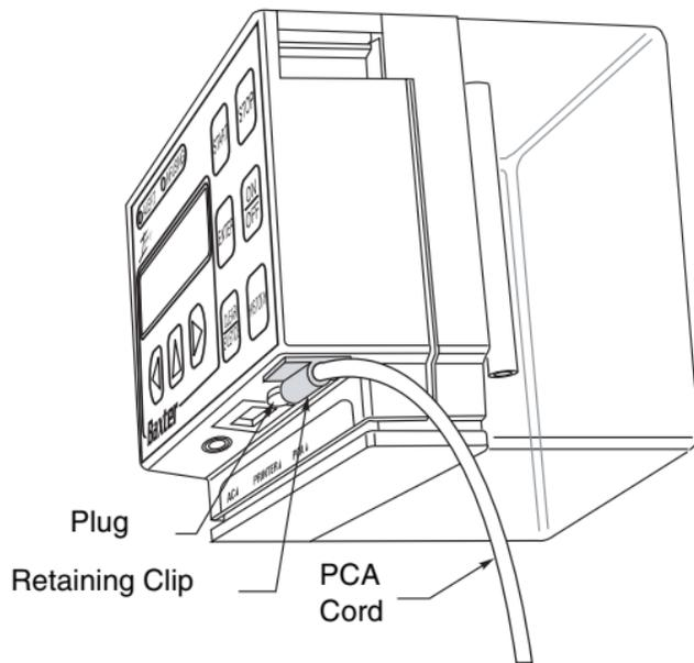
**Figure 3-4 Connected PCA Cord and Plug**
