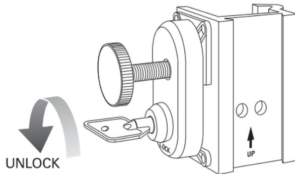
**Figure 3-12** *Unlocking the Clamp*
