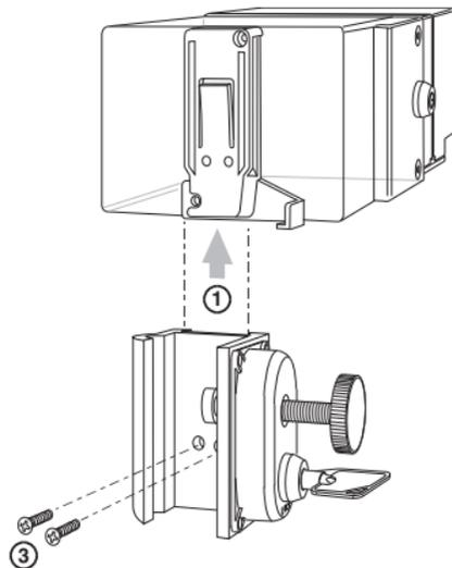
Figure 3-10 Attaching the Clamp
