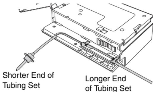
**Figure 3-8 Tubing Set Correctly Positioned**
