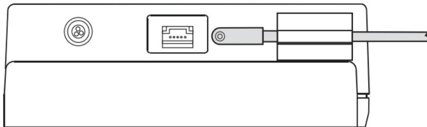
**Figure 3-3** *PCA Cord Connection Through the Retaining Clip*
