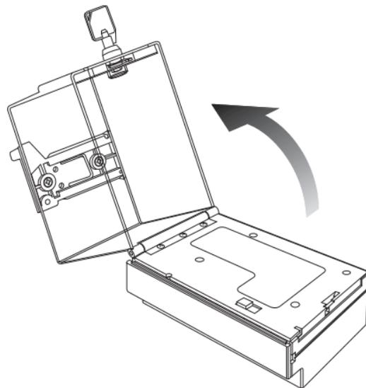
Open the cover with the pump face down.
