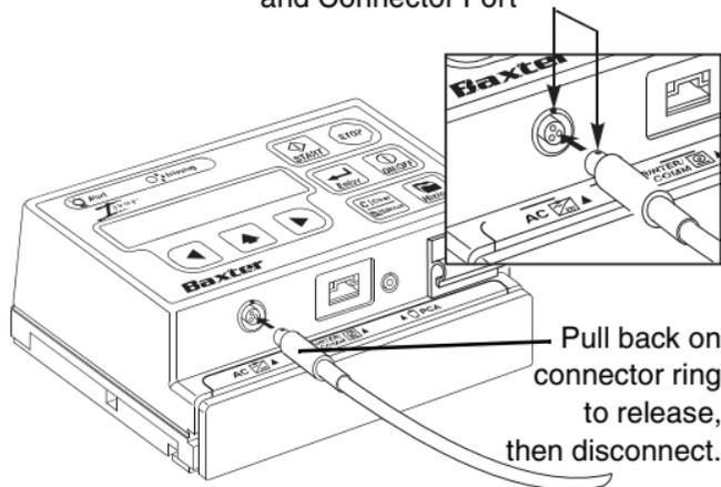
**Figure 3-2 AC Adapter Connection**
