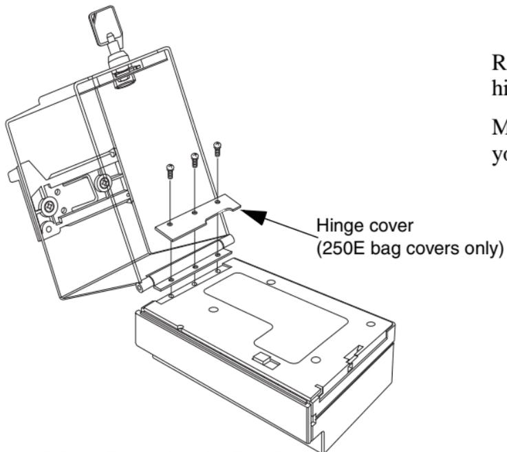
Remove the three screws that secure the hinges.
