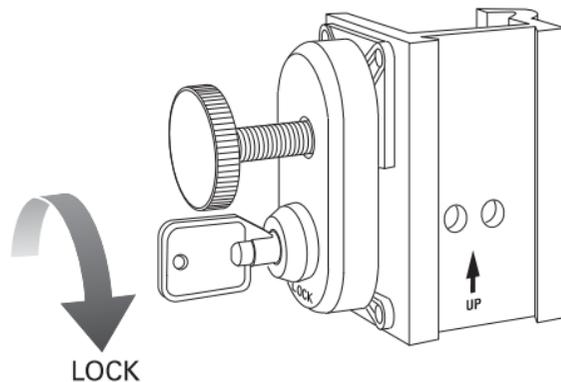
**Figure 3-11 Locking the Clamp**
