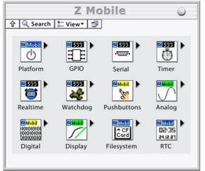
For this reason, the flexible standard platform "ZMobile" was chosen as device base for the construction of the handheld apparatus. Each of the above mentioned functions is already available as a tried and tested hardware and software component (Figure 4) and can be easily dragged and dropped from a palette into the program as shown in Figure 5.
