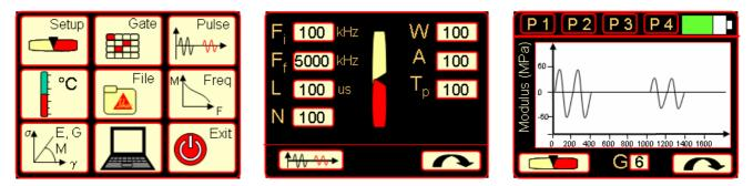
Figure 6. The clearly designed user interface with a main menu (left), parameter settings (middle) and signal graphics (right) conceals the complexity of the system
