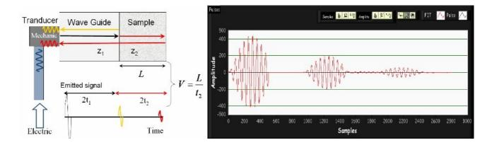
Figure 3. Left: an electric signal is converted to a mechanical signal with a transducer. The generated ultrasonic wave propagates through the material where it is submitted to a reflection at the interface between the wave guide and the sample. Right: the time of fly is acquired with the embedded oscilloscope.
