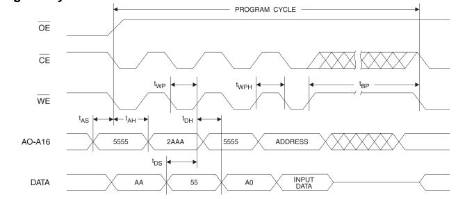
Chip Erase Cycle Waveforms
