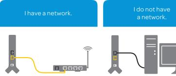
1. Connect the yellow Ethernet cable from the "Ethernet" port on your MicroCell to your router.
