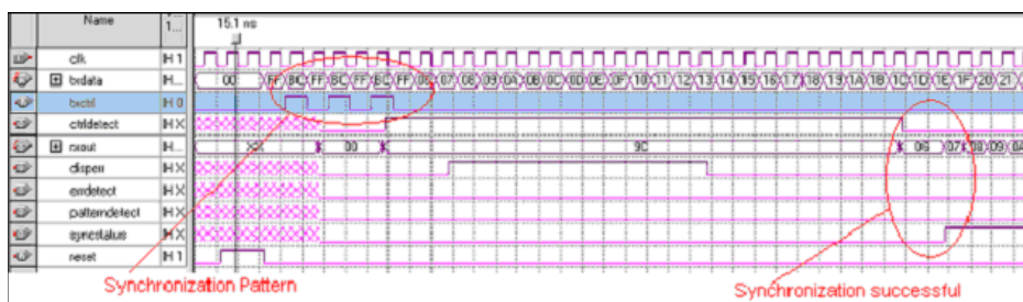
Figure 6–35. GigE Synchronization Sequence Quartus II Software Simulation Results
